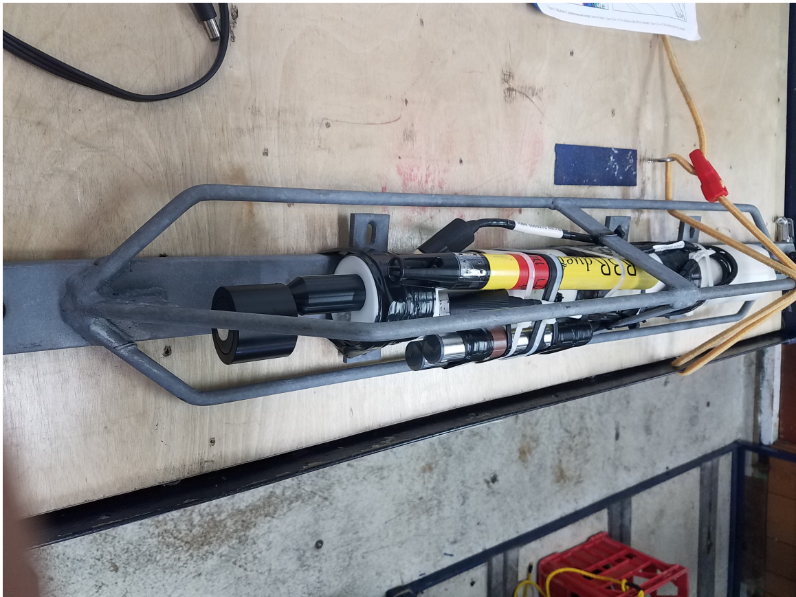
Figure 37: The uCTD package, comprised of a RBR Concerto with fluorometry sensors sampling at 6 Hz and an RBR Duet (temperature and pressure sensors) sampling at 16 Hz, both encased in a steel crash guard and attached to the fishing reel line through a small swivel.
