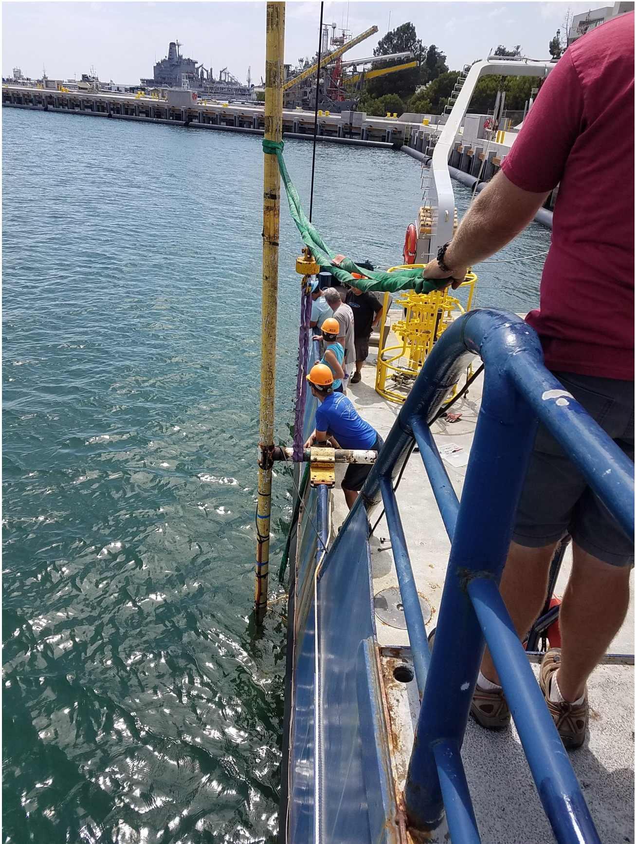
Figure 35: Metal pole mounted on the starboard beam for the 1200 kHz ADCP.
