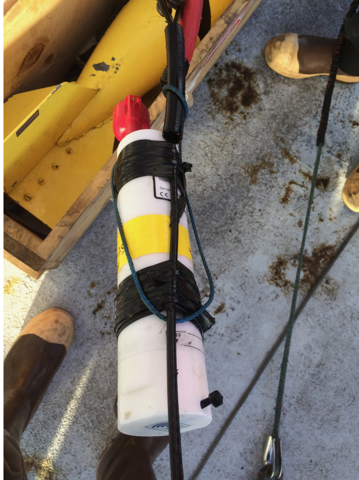
Figure 26: RBR Concerto 60381 upon recovery of Deployment 3 with the blue weight line wrapped between the instrument and the cable. The red conductivity sensor was found loose and easily rotating. Photo credit: Kate Adams.
