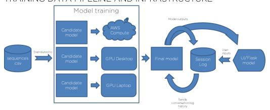
Production infrastructure is comprised of two Flask applications. The first is a rest API that ingests a dialogue history and impersonation value ("Monica", "Ross", etc.) as a JSON file. Essentially, it exposes the model. This API runs in the inference environment on an AWS instance. The second application is the user front-end chatbot. This can run on any machine in our flask environment. The chatbot app collects user dialogue,
