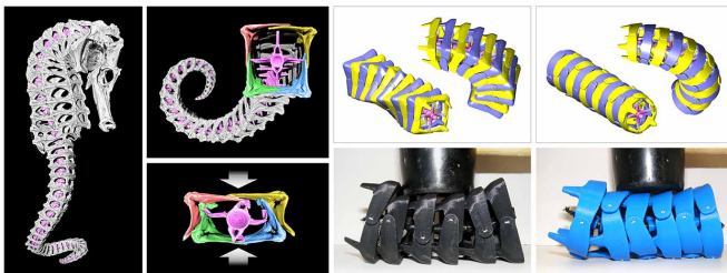
Left: seahorse skeletons are composed of highly articulated bony plates that surround a central vertebral column. Right: Bending and twisting performance of 3D printed prototypes.
