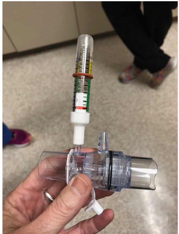
Dr. Sidney Merritt displays an in-house pressure measurement device, currently in testing for use on a system designed to split a single ventilator to serve up to four patients.
