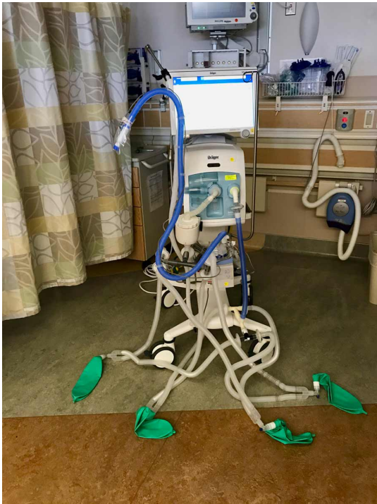
Using 3D-printed parts, Dr. Sidney Merritt and a team at the U.S. Navy and Lockheed Martin are developing a system to convert ventilators designed for a single patient to be used by up to four patients at a time.
