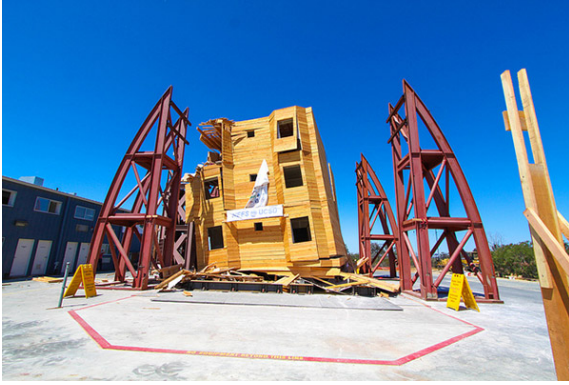
Engineers shook to failure a four-story wood frame building at the UC San Diego shake table on Aug. 17, 2013.
