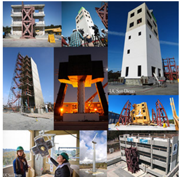
The UC San Diego shake table has been used to test a wide variety of structures. Clockwise from center of top row: a five-story building equipped with non-structural components (two pictures), a soft-story wood frame building, a precast concrete structure, a wind turbine, interior of the five-story building's surgery suite, a seven-story building, a three-story masonry building and a bridge column (image at the center).
