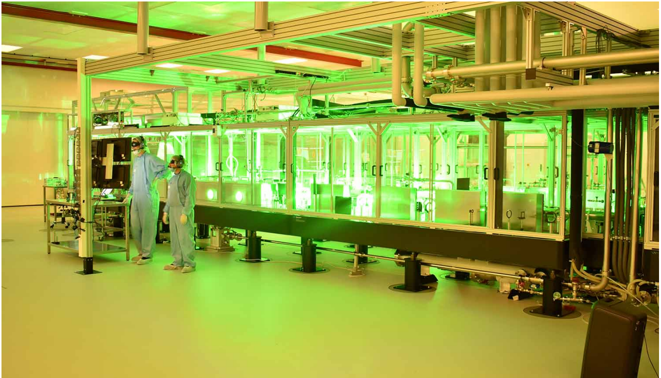
The study offers a recipe for researchers at the Extreme Light Infrastructure (ELI) high-power laser facility to follow to produce matter from light. Pictured is the L3-HAPLS advanced petawatt laser system at the ELI Beamlines Research Center. Photo courtesy of Lawrence Livermore National Laboratory.
