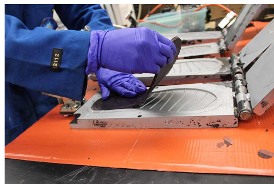
Foot-bed of flip-flops being pulled from a mold. Photo courtesy of Stephen Mayfield, UC San Diego.
