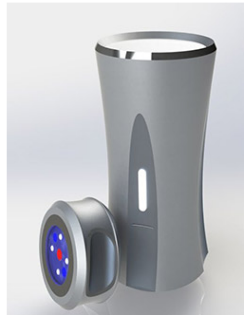
The prototype design of SENSE has two parts. The smaller piece samples temperature, heart-rate, and other vital signs. The larger piece can test water for heavy metals like arsenic and eventually bacteria and viruses.
