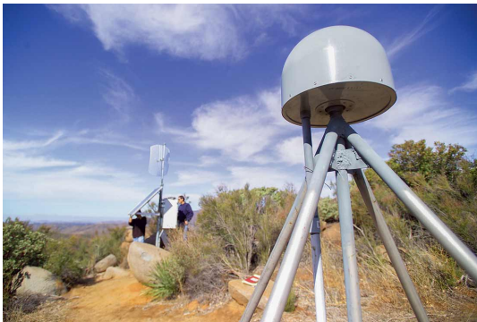
A GPS monument in San Diego County is part of the California Real Time Network that provides geospatial information throughout the state. The data is used to determine where ground movement has happened after an earthquake.
