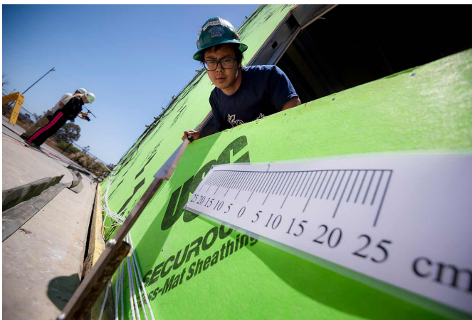
A structural engineering Ph.D. student checks a gage to see how much a building has moved during a test on the shake table.
