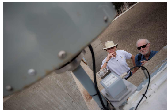
A team of researchers from across UC San Diego are using lasers, GPS sensors and drones to create a digital record of Geisel Library that will serve as a baseline health assessment in the event of an earthquake.
