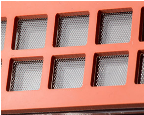
image of the 12-nanoliter-volume microwells in which amplification is confined in the new single-cell sequencing approach called Microwell Displacement on System (MIDAS).
