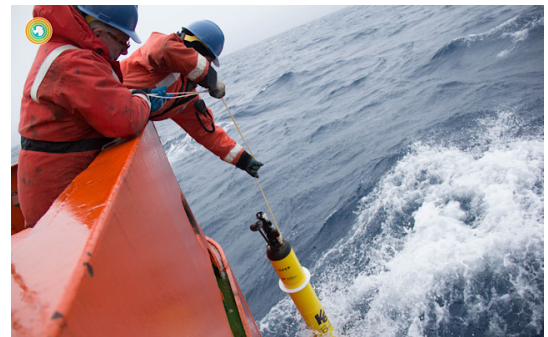
Deployment of a biogeochemical float. Photo: SOCCOM Project
