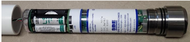
39plus with embedded thermistor and external RS-232 connector; detail similar for other configurations
