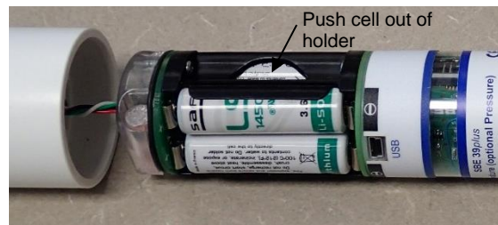
39plus with external RS-232 connector; battery detail similar for other configurations
