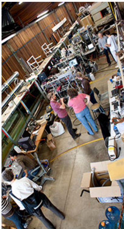
Researchers surround a 33-meter (108-foot) wave tank at the Hydraulics Laboratory at Scripps Institution of Oceanography. The wave tank creates a closed environment that allows researchers to control studies of air-sea interactions and of aerosol formation and evolution.
