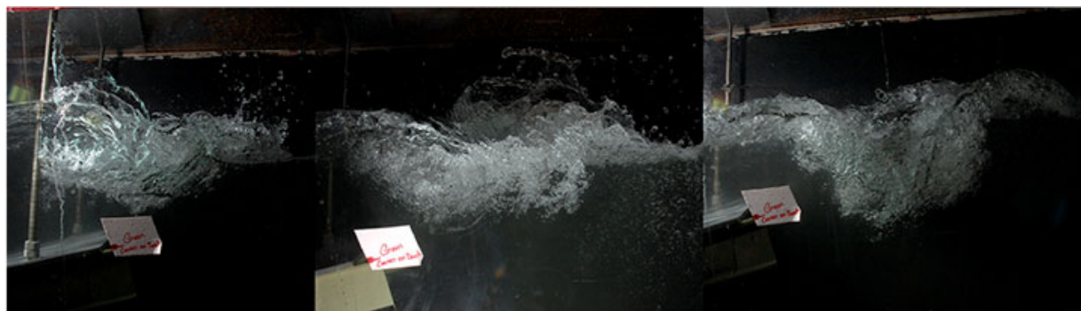
Breaking waves inside a wave tank that houses a replica ocean-atmosphere system for a CAICE lab experiment. The mechanically generated waves simulate in a controlled setting ocean processes that eject aerosols into the atmosphere.
