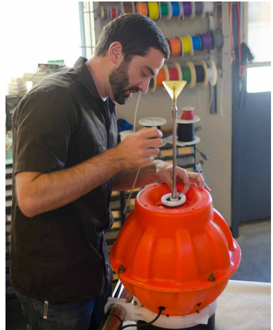
Scripps Oceanography development engineer David Black assembles a Deep SOLO instrument, designed to augment ocean measurements in the global Argo network.
