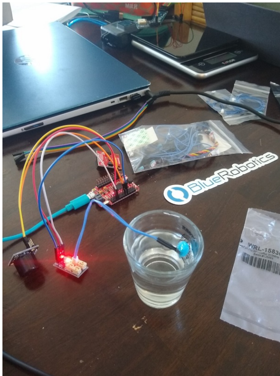
A cheap, durable flooding sensor designed by the CCCIA-sponsored team in the Hacking for the Oceans class.
