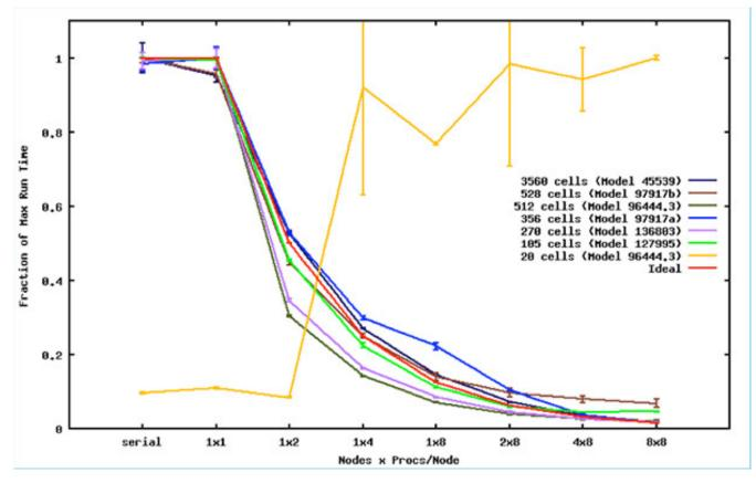
simulation time (Y axis) decreases for larger models as more processors (X axis) are used. The models are available from ModelDB which has large collection of computational neuroscience models. The results were generated using the NEURON simulation software on SDSC's Triton cluster. Image courtesy of Subha Sivagnanam and Kenneth Yoshimoto, San Diego Supercomputer Center, UC San Diego.
