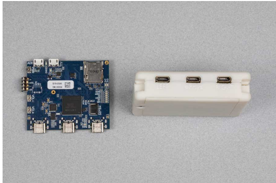
OSP's hearing aids research platform built with smartphone chipsets
