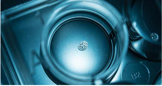
A 3D printed, two-millimeter implant used to heal severe spinal cord injury in rat models
