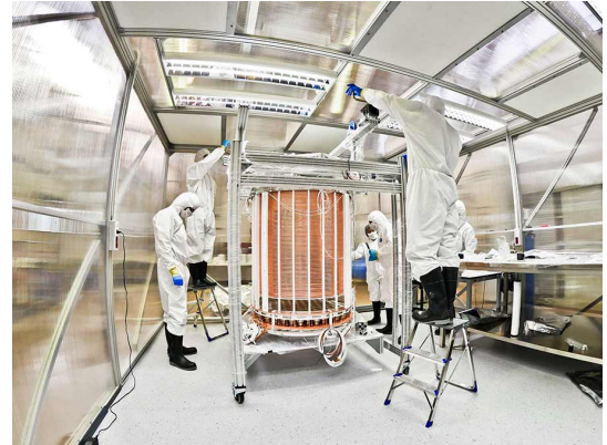
The heart of the project: The XENON1T Time Projection Chamber after assembly in a clean room. Courtesy of the XENON Collaboration
