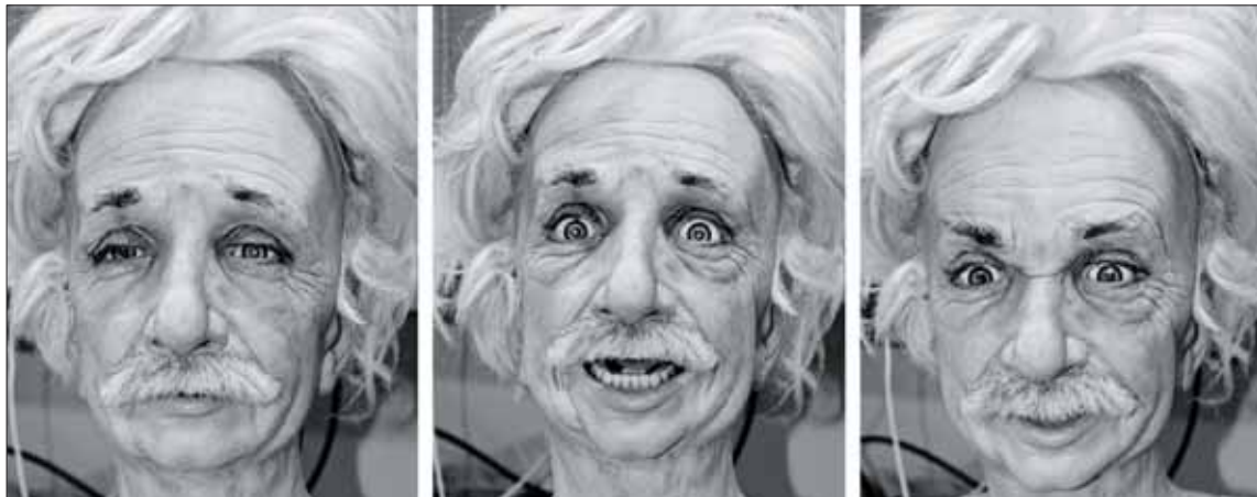
ERIK JEPSEN/GUARDIAN Facial-recognition software designed by Calit2 scientists allows the Einstein Robot to naturally interpret and mimic human facial expressions.
