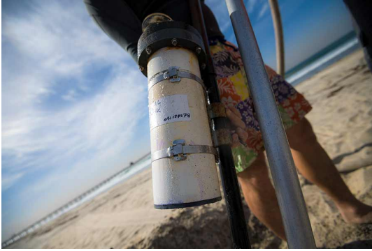
Three pressure sensors will be installed at the mean high-water line throughout Imperial Beach. The sensors will be retrieved after winter to collect and analyze the data. Photo by Erik Jepsen/UC San Diego Publications
