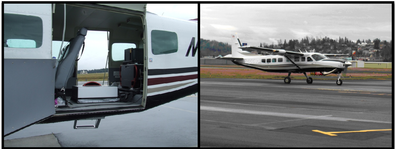
The Cessna Caravan is a stable platform, ideal for flying slow and low for high density projects. The Leica ALS50 sensor head installed in the Caravan is shown on the left.
