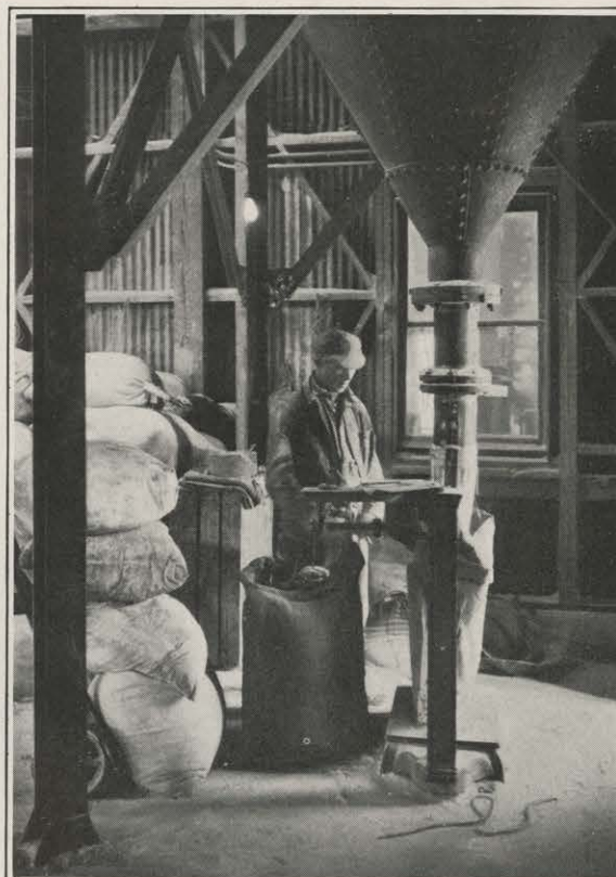
SACKING CALCINES TO BE SHIPPED TO REFINERIES.
