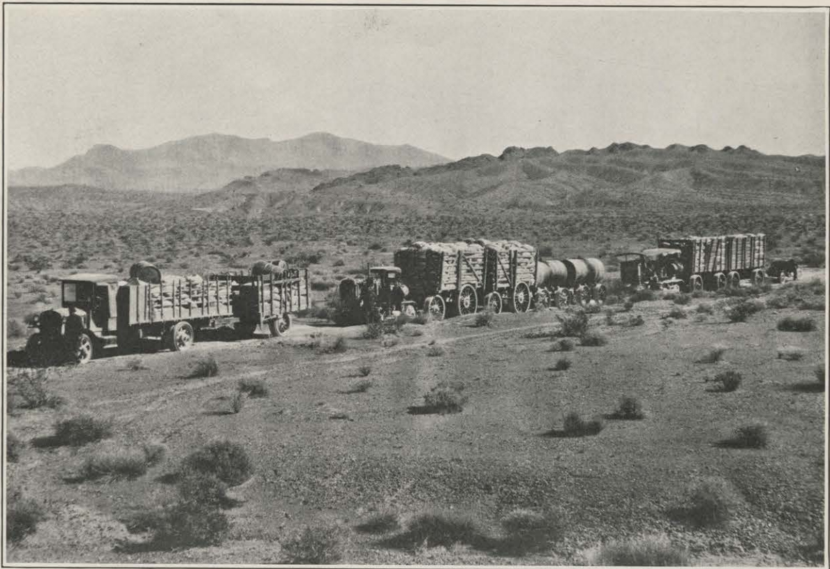
TRANSPORTATION TO RAILROAD—ONE MOTOR TRUCK AND TWO TRACTORS WITH TRAILERS CARRYING 50 TONS OF CALCINES AND TWO OIL TANKS.
