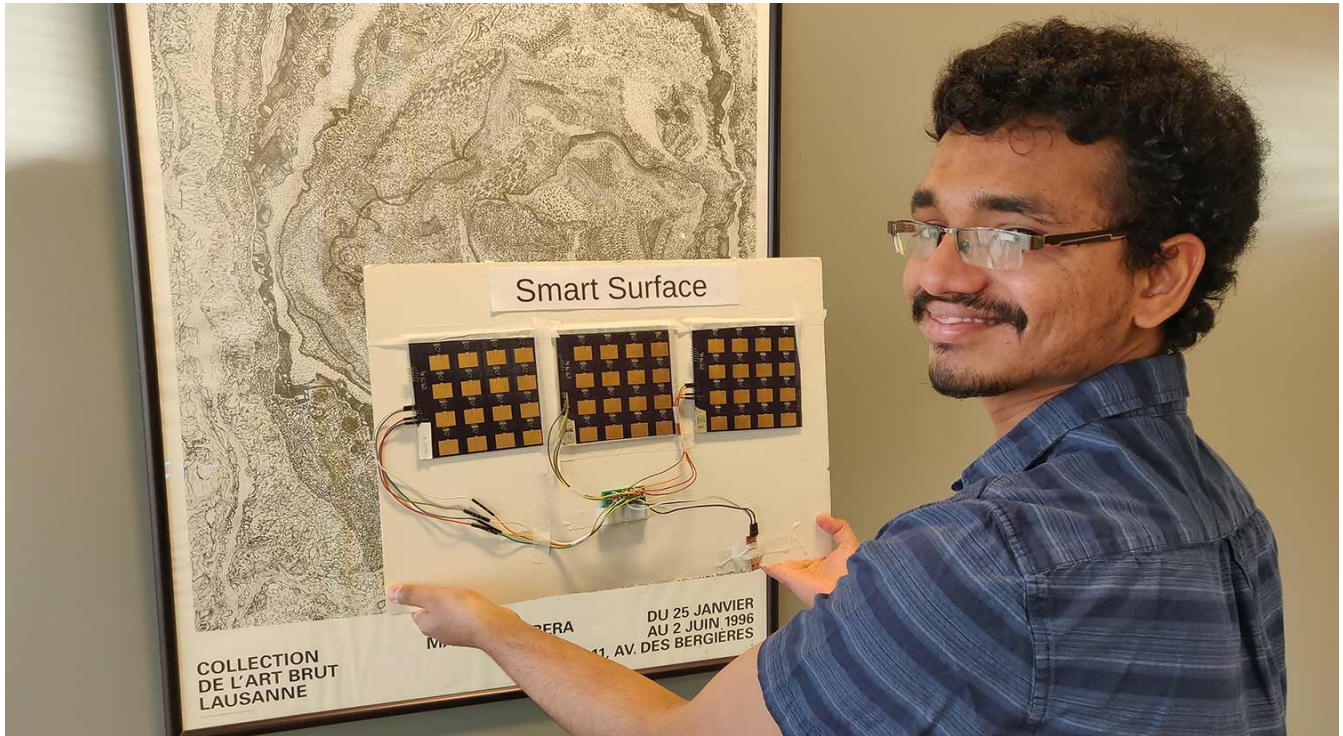
Manideep Dunna, a UC San Diego electrical and computer engineering Ph.D. student, holds a prototype "smart surface" that can be stuck on the wall to improve WiFi connectivity in the home and office.
