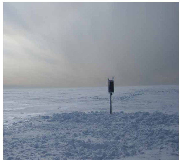
A seismic station that is part of a 34-unit network across the Ross Ice Shelf. Scripps oceanographer Peter Bromirski and colleagues installed the network to study the vibrations from ocean waves that could cause the shelf to crack and eventually drift away from Antarctica.
