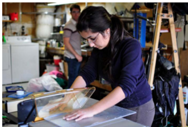
Mehria Sayad-Shah cuts Lexan panels for the fluid containment portion of the device.
